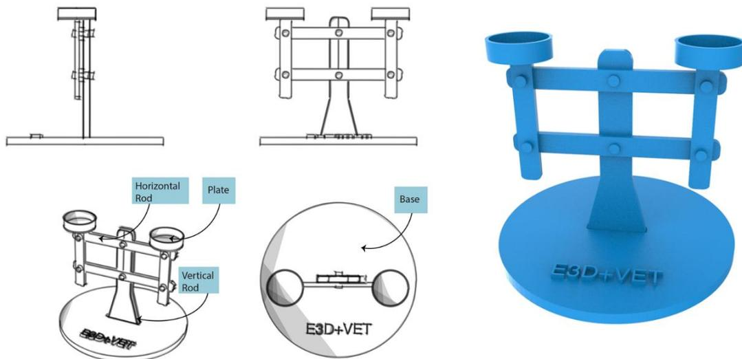
**Figure 2.** Balance design in different perspectives (left) and the 3D printed model (right).
